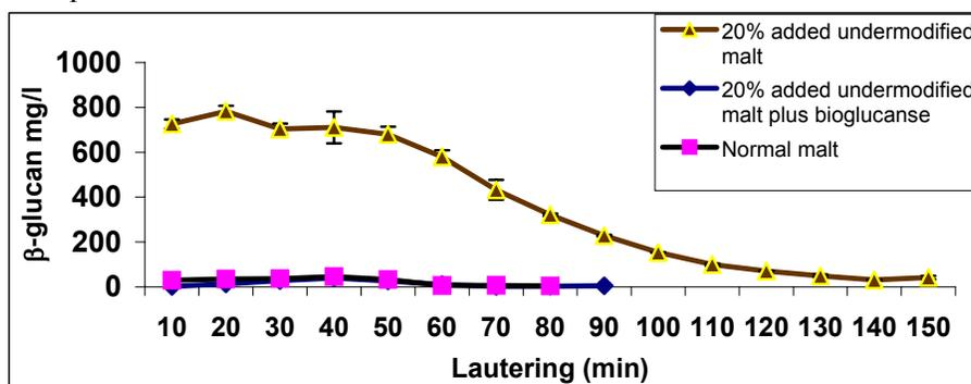
**Figure 4.** Effect of bioglucanase on the beta glucan content of 20 % added under-modified malt. The  $\beta$ -glucan content can be compared to that of the normal malt lauter run and to that containing 20% under-modified malt with no added bioglucanase. Bioglucanase was added to a mash concentration of 1300 U/l. Samples were assayed in duplicate.
