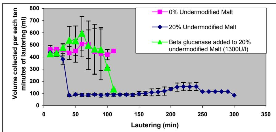
**Figure 5.** Effect of bioglucanase on the lauter run off time of malt mashes containing 20% added under-modified malt. The effect of reduced  $\beta$ -glucan content on run off times in the lauter tun can be seen when compared to the 20% added under-modified malt run without added bioglucanase.
