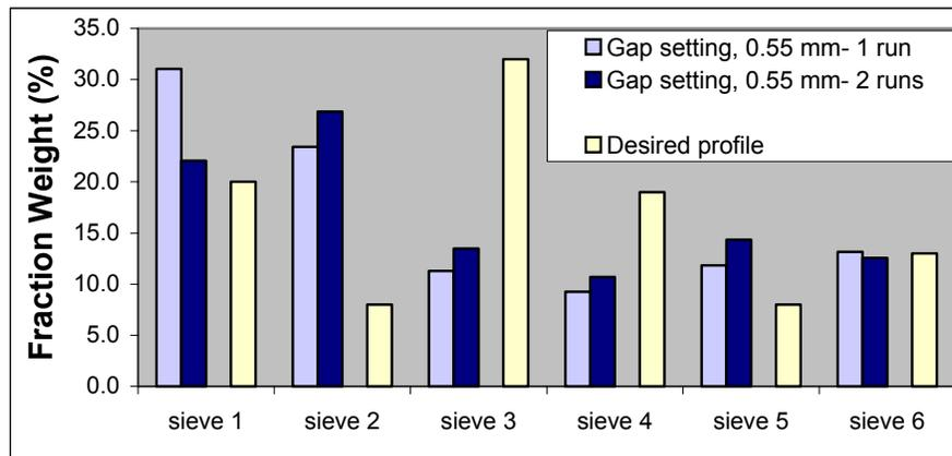
**Figure 2.** The effect of multiple runs through mill on grist particle size distribution at 0.55mm gap setting.
