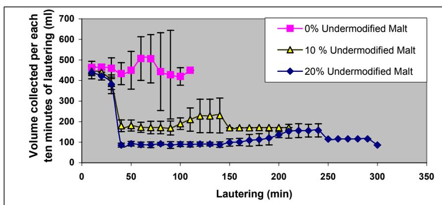
**Figure 3.** Comparison of wort volume collected between lauter tun runs with 0, 10 and 20 % added under-modified malt. Volume shown is that collected during each ten minutes of lautering. Runs were done in triplicate
