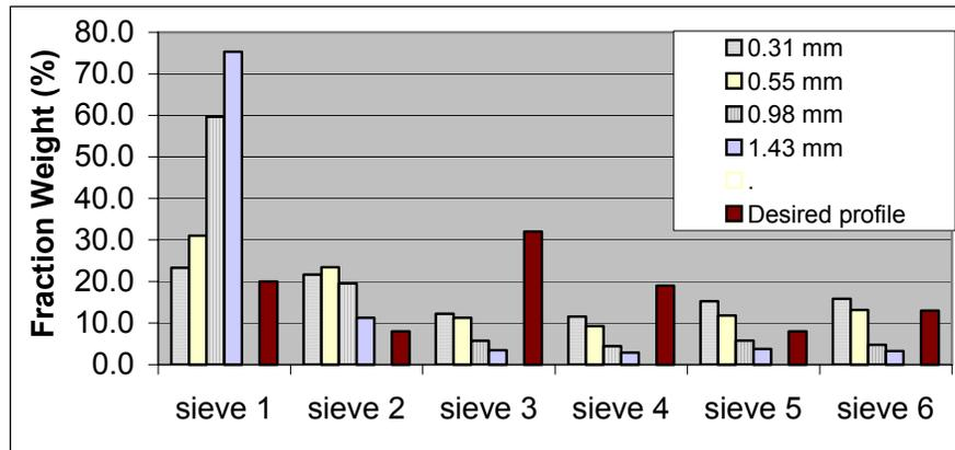
**Figure 1.** The effect of gap size, between the mill rollers, and grist particle size distribution. Sieving produces 6 fractions. Fraction 1 containing husk to fraction 6 containing fine flour.
